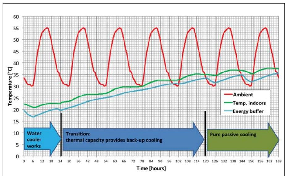
Fig. 4. Testing verified the shelters' intrinsic ability to deal with the failure of active cooling systems.
