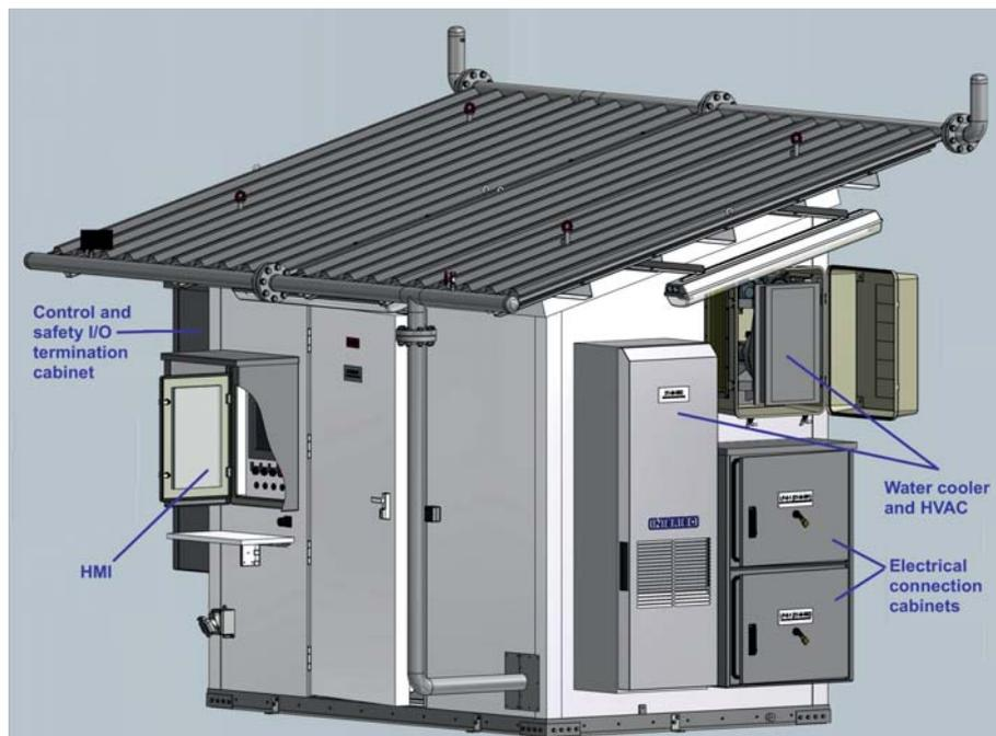
Fig. 2. Intertec’s ‘peri’ shelter design features a novel inside-out construction style, with all elements for installation and normal operation accessible from the exterior. The actual shelter can be seen in Fig. 1.
