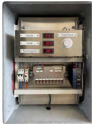
The basic VARICOOL setup includes a compressor, an external and an internal heat exchanger, the latter of which actively cools a steel plate, which in turn acts as a thermal buffer. The instrumentation or electronics are then mounted to the buffer using C-rails.
